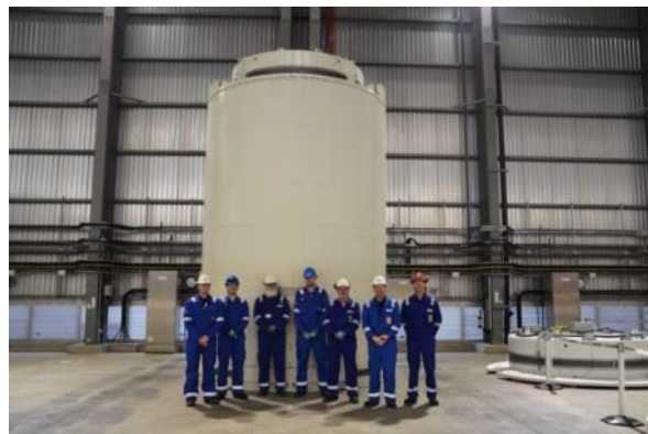
Figure 17: HI-STORM MIC spent fuel cask in place in Sizewell B power station Store. Radiation is contained to a level that it is safe to work around and even touch the casks. (Image: Holtec)
