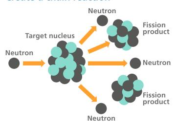
When the nucleus of a uranium atom is hit by a neutron it splits into two. This is the process of **nuclear fission**.
